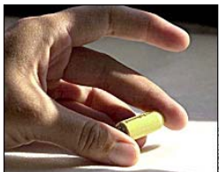
Figure 1. A wireless endoscopy system in a capsule provides real-color images of the GI tract after the patient swallows the device.
